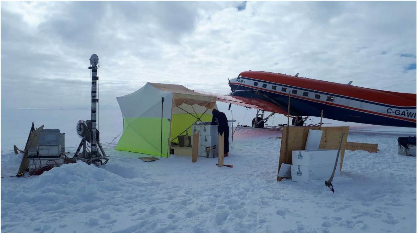
Drill camp of the airborne campaign in Northeast Greenland, 2019, with the field team participations. A similar setup is planned for the ICELINK drilling campaign. Left: Drilling rig on a Nansen sled, center: Logging tent, right: Parked Basler/Dornier aircraft.
