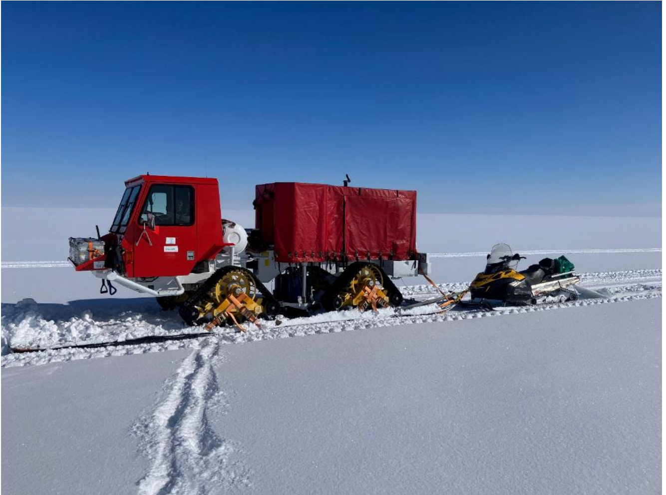
AWI's VibroSeis truck during a measurement campaign in Antarctica in 2024/2025. Photo credit: Olaf Eisen.
